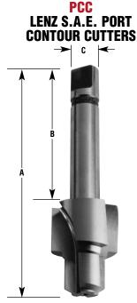
These tools have three flutes which form the standard internal O-Ring Boss for straight thread tube fittings. Standard in high-speed steel. Carbide tipped available on special order. Four flute cutters available on special order.
