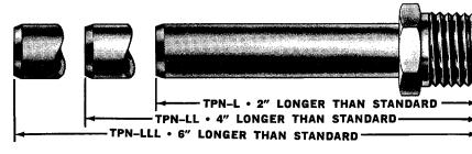
Example of L, LL, and LLL Part Numbers-Where a 12TPN with an overall length of 6%/6" is desired, request 12TPN-LL (4" longer than standard 2<sup>9</sup>/16")
